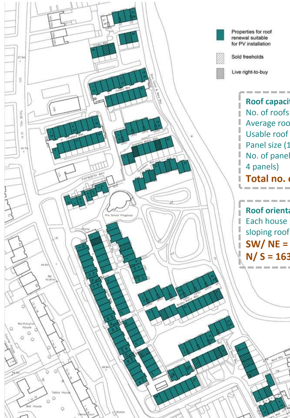
Roof spaces suitable for PV installation
