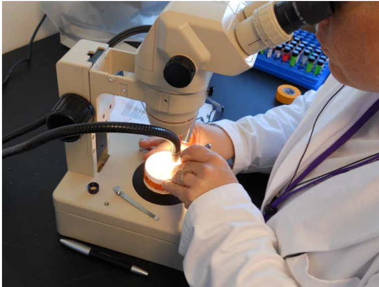
Figure 12. Microplastic fragments are extracted from the prepared sample during a microscope examination.
