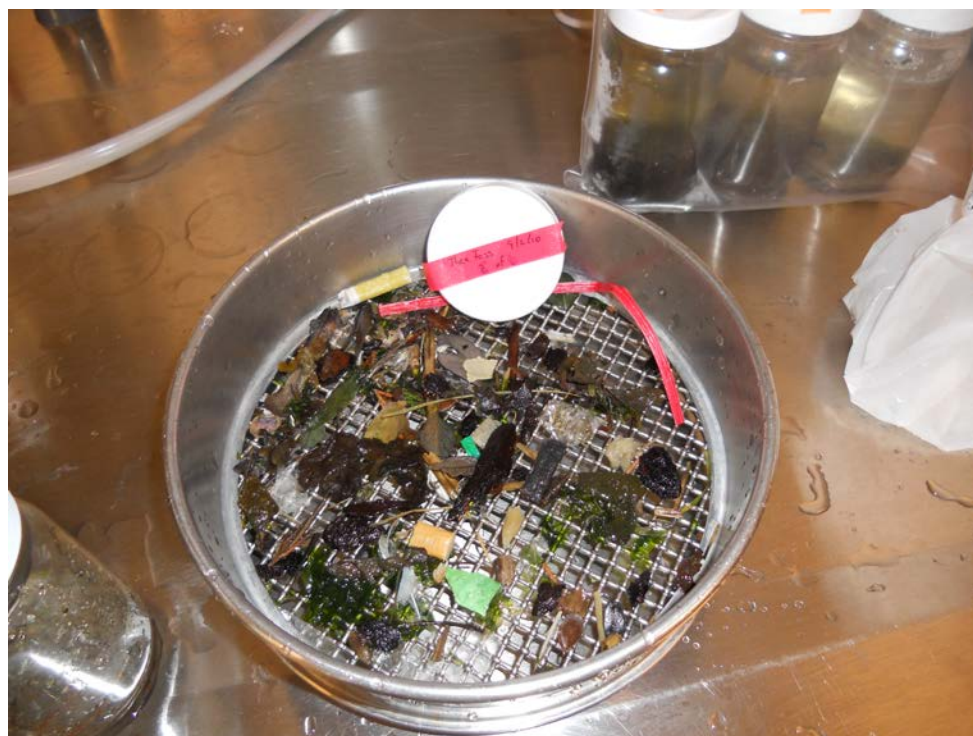
Figure 4. Sieving and rinsing field samples.
