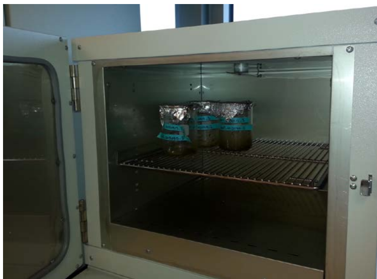
Figure 6. Sieved samples are dried in an oven to determine dry weight.
