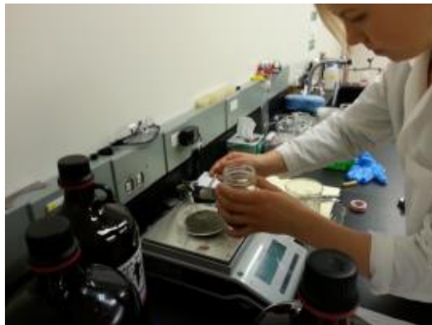
Figure 15. A beach sand (or sediment) sample is weighed.
