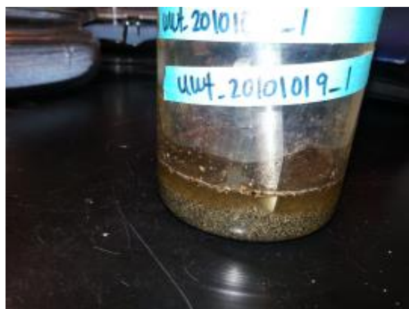
Figure 16. Lithium metatungstate is added to a sediment sample.
