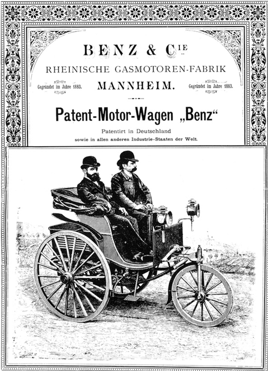
Figure 2.11 Cover illustration of the first (1888) catalogue by Benz & Cie. is a slightly modified version of the three-wheel vehicle that was patented and publicly driven for the first time in 1885. Photograph courtesy of DaimlerChrysler Classic Konzernarchiv, Stuttgart.
