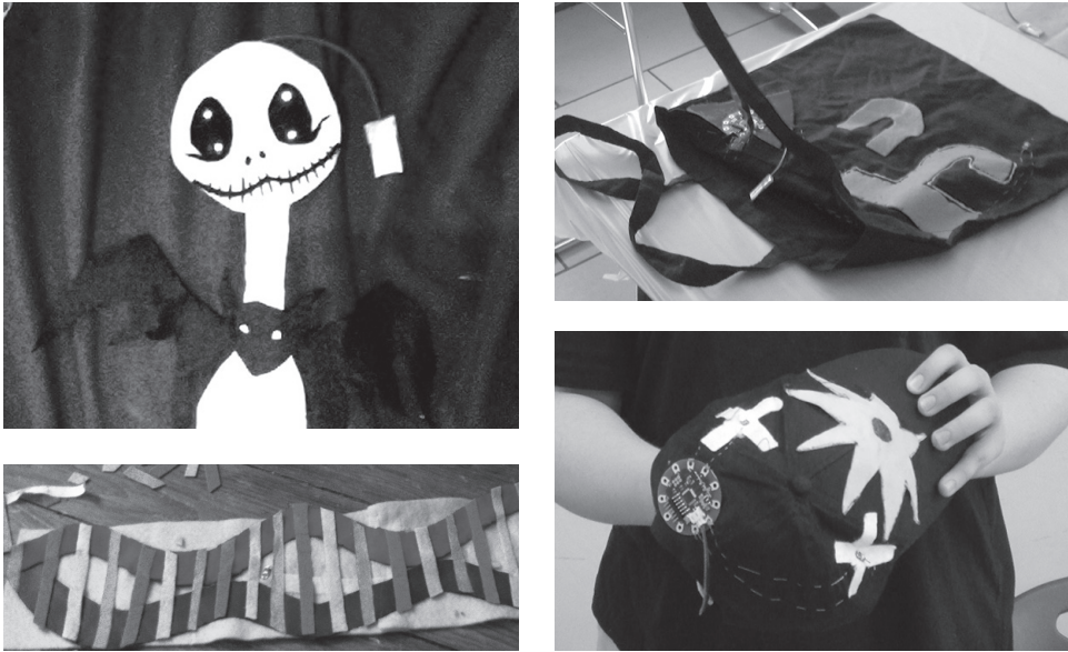
Image 2. Students' final e-textile designs: a Jack Skellington patch with light-up eyes decorates a backpack (upper left); a tote bag with light-sensing handles (upper right); a wearable belt with a double-helix (lower left); and an anime-inspired hat (lower right). Photographs copyright © Kristin A. Searle
